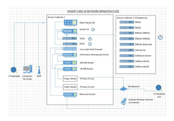
The telephony server equipment is housed onsite at the Urgent Care 24 headquarters premises in Wavertree. All I.P handsets have to be configured on the primary and secondary Mitel Controllers (PBX01/2)
